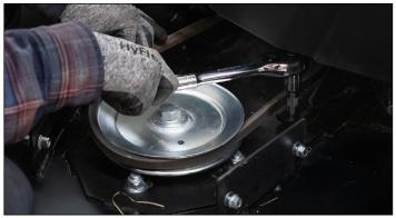
**QUICK BELT CHANGES** Don't worry about changing the deck belt, with a breaker bar or ratchet you can easily use the tensioner arm to adjust and replace the belt.
