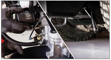
**TOOL-FREE OIL CHANGES** No need to get on the ground or raise your mower to change the oil with the tool-free oil drain extender and easy to remove oil filter.
